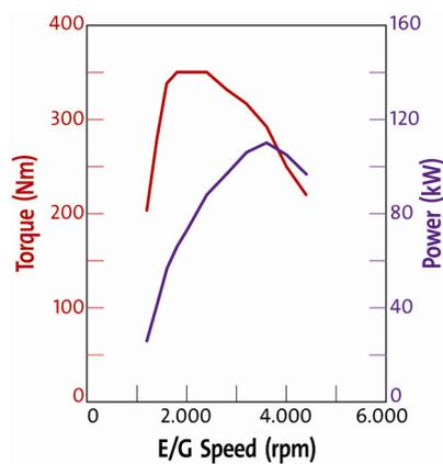
2,0 litros, 4 cilindros DOHC turbo DIESEL
